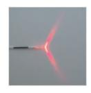
CORONA 360 600 Fused Fiber® delivers a homogeneous pattern directly to the vein wall without front-firing.
